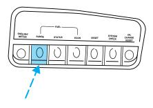
For maximum accuracy of this display feature, the ignition should be in the OFF position during fueling. The display FUEL LEVEL ERROR indicates a problem with the fuel indication system. See your dealer or qualified service technician for system maintenance.
